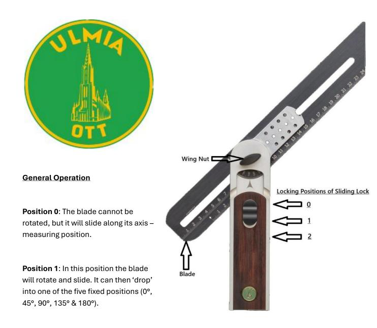
**Position 2**: In this position the blade will rotate and slide, but it will not 'drop' into one of the fixed positions. This allows you to select any angle and then lock the blade using the wing nut.
