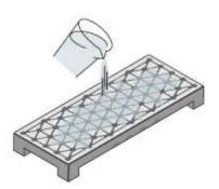
Place the NAORU lapping plate somewhere stable. Apply enough water to permeate the whole plate. If any water is left on the surface, the powder may get washed away.
