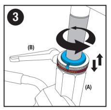
Allow the sealing disc and TRAC to sit onto the stem colum (A) and adjust to the required height by rotating the outer ring. Now position the tool rest in the desired position and lock the stem in the normal way with the lathe locking handle (B).
