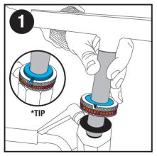
Place the TRAC & seating disc onto the stem.
