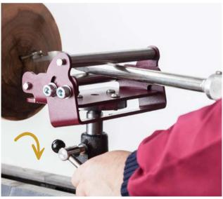
Place the desired tool onto the lower roller and adjust the height of the stem in the banjo, so the cutting edge of the tool is at the required position and lock the stem into place
