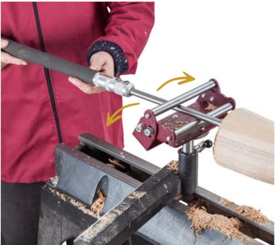
The rollers allow the user to move the tool lightly from left and right whilst being held securely
