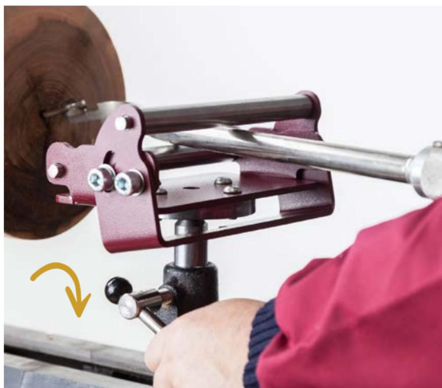
Place the desired tool onto the lower roller and adjust the height of the stem in the banjo, so the cutting edge of the tool is at the required position and lock the stem into place
