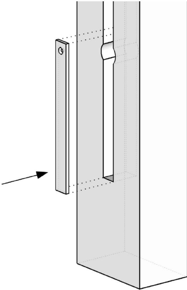
Install the bearing plates into the leg and the chop at the bottom of the mortises. They should slip into the mortise easily and rest on the end of the mortise and flatly on the bottom. Make sure you don't trap any wood shavings or chips behind the plate. The plate needs to be flat to the mortise bottom. Position the countersunk hole at the top, pre-drill, then drive the included wood screw to secure the plate.
